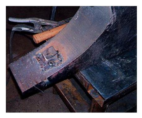
This view shows the short length of 1-1/2" X 1-1/2" thin wall steel tubing that was used to bring the bottom of the Hardie Hole flush with the bottom of the heel.
