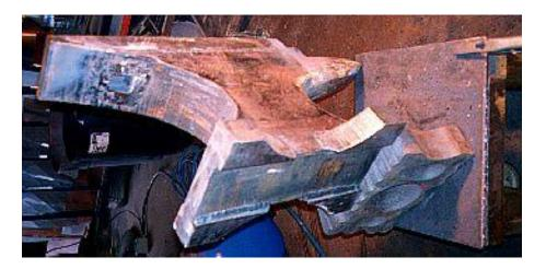
View showing the finished second pass of the hard facing with more edge buildup. Notice how the hardie hole sticks up through all the hardsurfacing.
