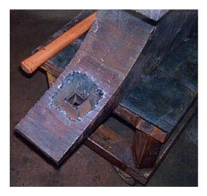
Drawing showing construction of the Hardie Hole Box and the hole cut in the anvil. Be certain to cut enough from the underside of the anvil to allow solid welding of the box throughout the anvil heel. \_\_\_\_
