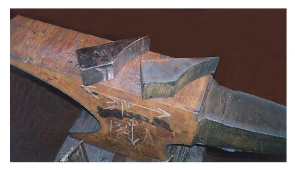
After you have the cut blank profile, you have to do a couple of bevel torch cuts by hand to give the shape to the horn.
