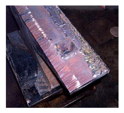
The edges are the hardest parts to build up due to the high amperage of the weld, so many smaller beads will be needed to build these up to the point that they can be ground off to a square edge.
