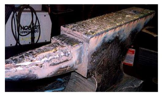
When hard facing the sides, I go about 1-1/2" down and run a simple bead to act as a guide.
